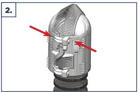
2. Route the conductor out the seam of the Guard at the small fingers. Close the Bushing Guard so that the two loop latches fit into the opposite half's square receptacles.
